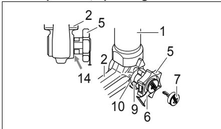
**Unlocked position, ball bar not mounted**
